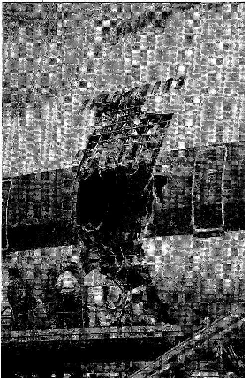
Fuselage of 747 after cargo door blew off, killing nine people.
