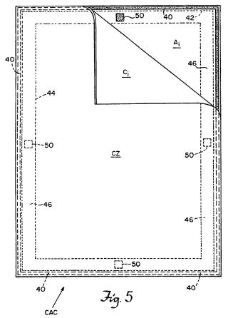
Surface  $C_i$  is the protected inner surface of the copper foil;  $A_i$  is the inner surface of the aluminum substrate. A band of flexible adhesive 40 joins the substrate and the foil at the edges, creating a protected central zone CZ. The specification explains:
