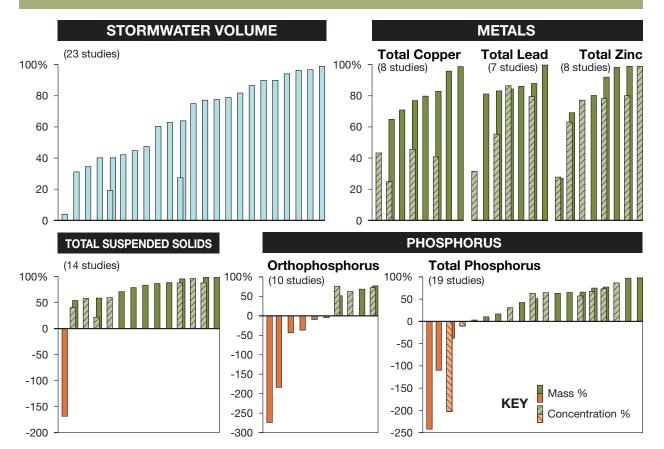
Stormwater volume and pollutant reductions reported for bioretention systems vary widely. (See the full report for a detailed explanation and data for additional pollutants.)
